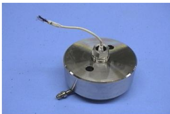
Figure S3. Photograph of an electrochemical cell.
