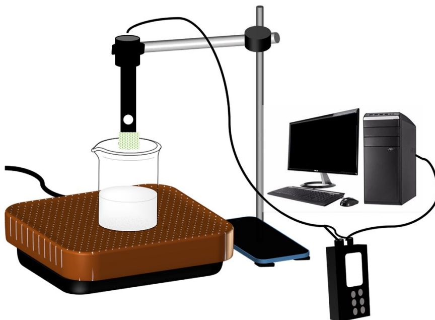
Fig. S1 Oil spillage monitoring system based on oil oxygen detecting probe sealed in hydrophobic and oleophilic porous materials with paraffin film, schematic of the oil spillage online monitoring system.
