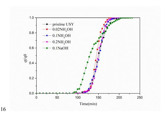
**Fig. S2** Breakthrough curves of all studied samples under humid condition (RH=30%).
