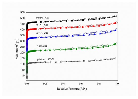
15 Fig. S1 Nitrogen adsorption-desorption isotherms of all studied samples.
