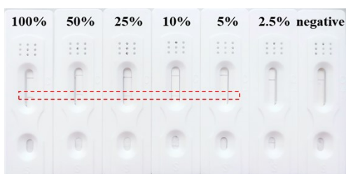
Figure S2 The pregnancy test paper was constructed with ENC-2 membrane to detect different dilutions of positive urine samples and negative urine samples
