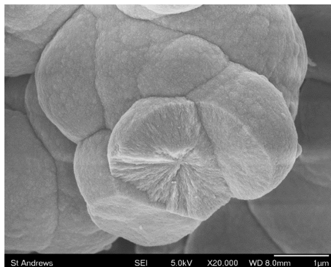
Fig. S2 High resolution SEM image of Mn(0-24). The broken spheres show the dense and polycrystalline cores.
