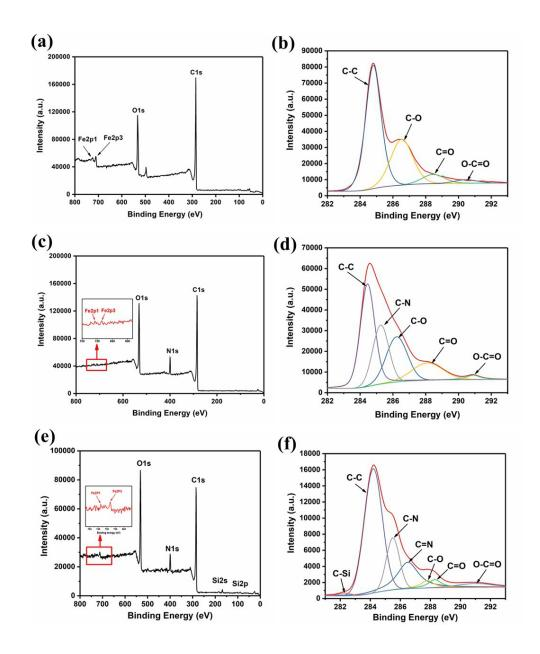
Figure S1 XPS wide scan and C1s core level spectra of (a and b) EGF, (c and d) GFA, (e and f) GFA+KH550
