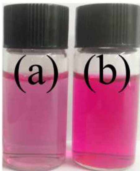
Figure S29. Photos of the dye solutions before (a) and after (b) absorption by D1 xerogel, respectively.
