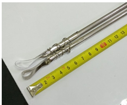
Fig. 1S The photo of the H + /H 2 , Ni made from nickel pipe and nickel foil employed in this study
