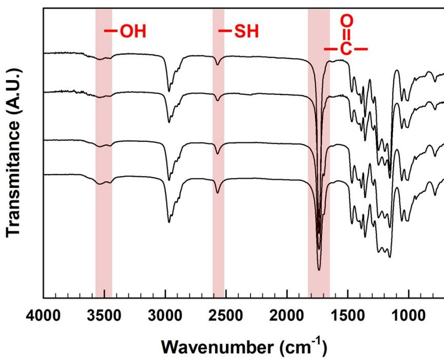
**Figure S3.** FT-IR spectra for crude product through direct esterification preliminary reactions (entry preEXP-1 ~ preEXP-4).
