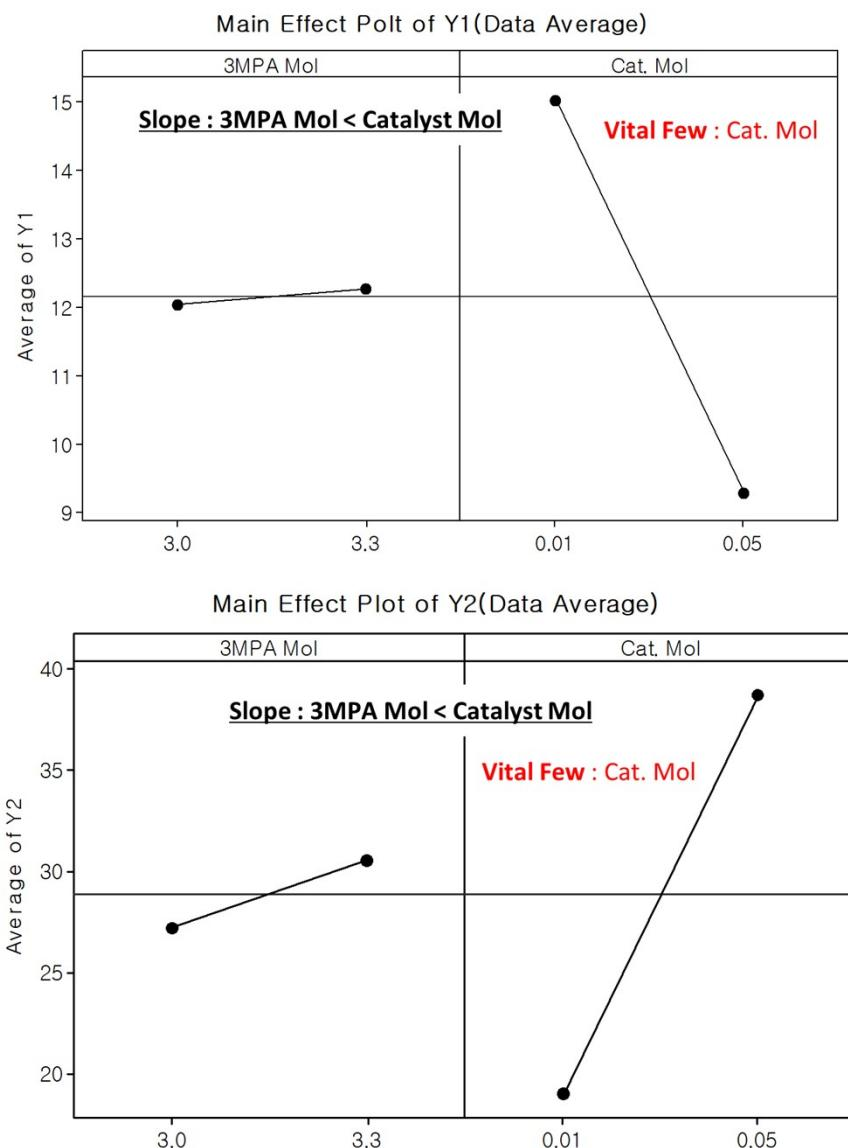
**Figure S4.** Synthesis parameters for the direct esterification reaction depending on reactant ratio and acid catalyst concentration.
