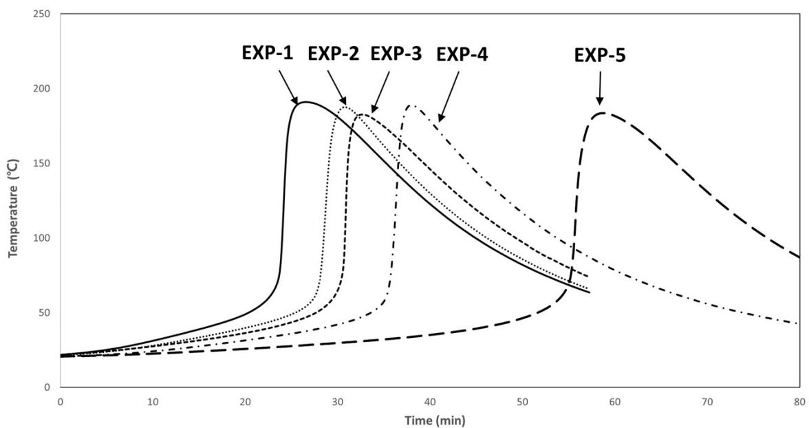
**Figure S5.** Thermograms corresponding to curing behavior for TMPMP-epoxy mixture with base catalyst.
