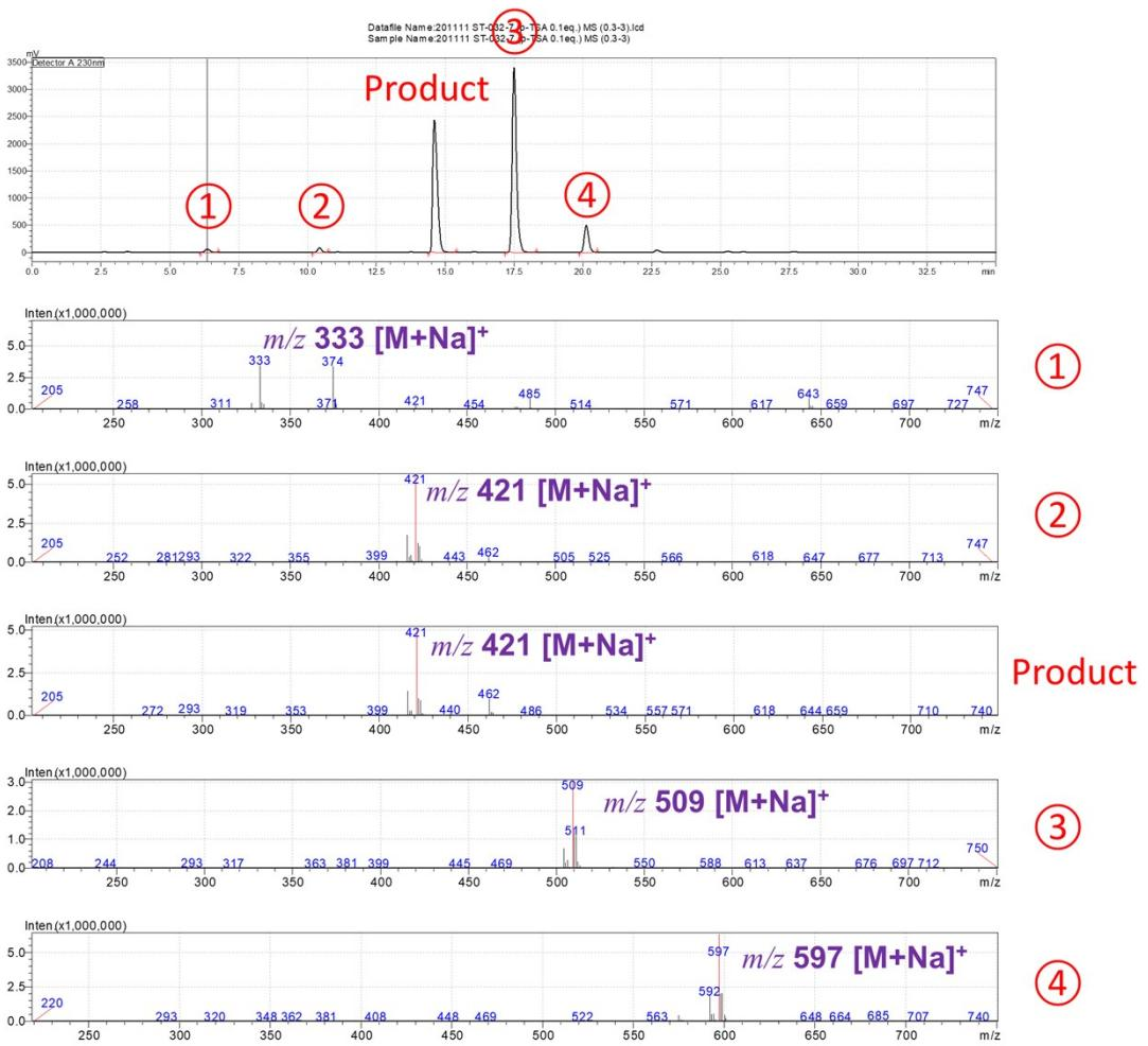
**Figure S1.** HPLC chromatograms and mass spectra for eluted peaks of TMPMP sample.
