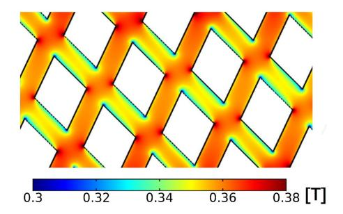
**Fig. S1.** Numerical simulation of the magnetic field distribution in the grid-like pattern. There is discrepancy in the distribution of the magnetic field in bar areas with different angles.
