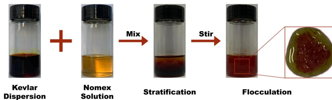
Figure S1. Process of mixing Kevlar dispersion and Nomex solution.
