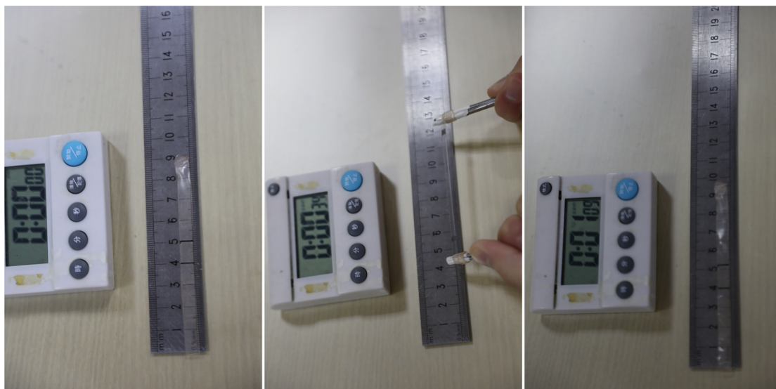
Figure S18. Optical images of PU-HM4-HP6 that can recover its original length after being stretched to 650 % strain
