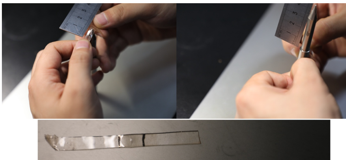
Figure S19. Optical images of PU-HM4-HP6 that can tolerate puncture
