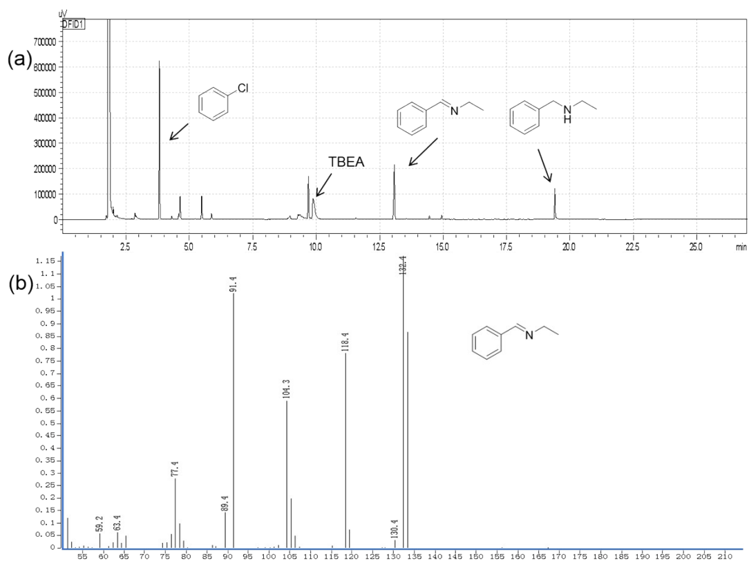
Figure S13. (a) The GC analysis of product (Table 2, entry 11); (b) The MS spectrum of product (Table 2, entry 11).
