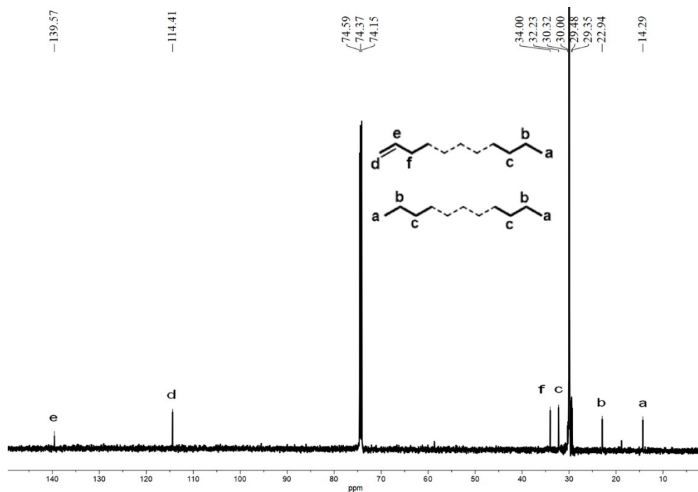
Fig. S4 13 C NMR spectrum of the polyethylene sample generated using Co4 /MAO (entry 7, Table 2); recorded in tetrachloroethane- d 2 (δC 74.37).
