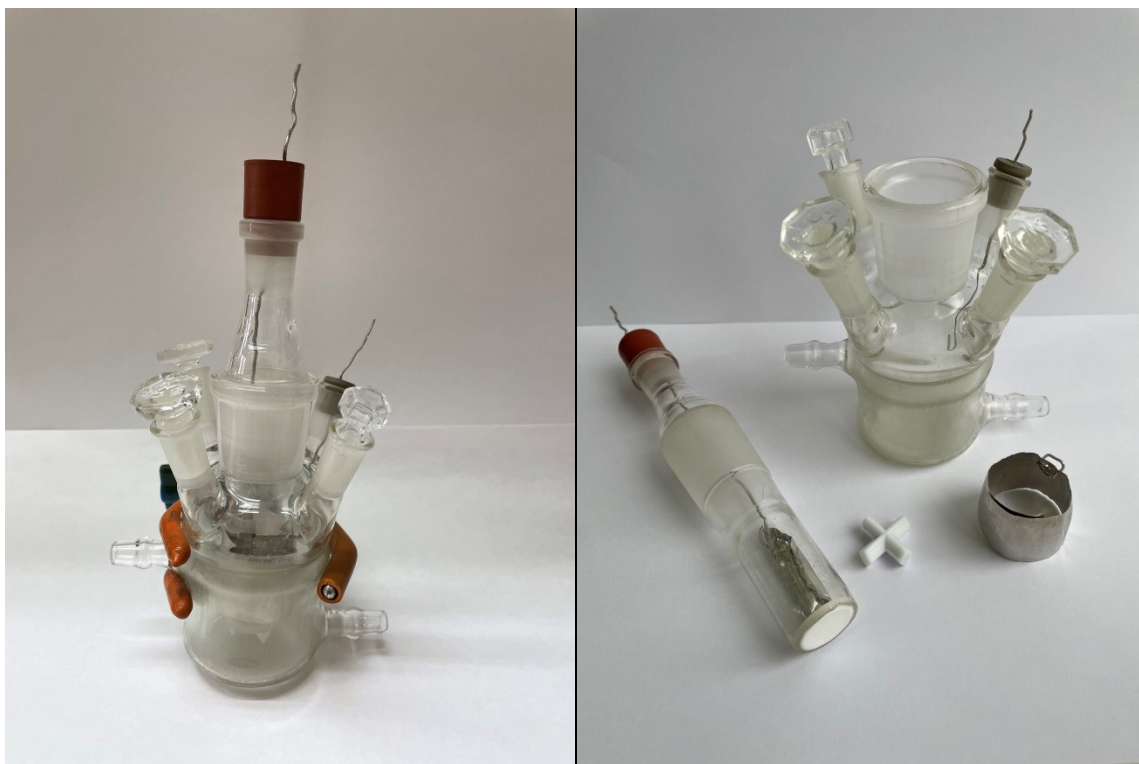
Figure S1. Electrolysis setup: cylindrical cell with divided anodic and cathodic compartments. The ceramic plate with the pore size of 900 nm is a membrane, the cylindrical platinum with a surface area of 20 \text{cm}^2 is cathode and the platinum rod is anode. The cell can be thermostatted.
