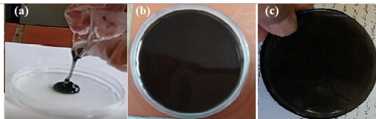
Fig. S6 The preparation process of the hydrogel films. (a) Pouring primary gel into a Petri dish, (b) molded hydrogel and (c) hydrogel film.
