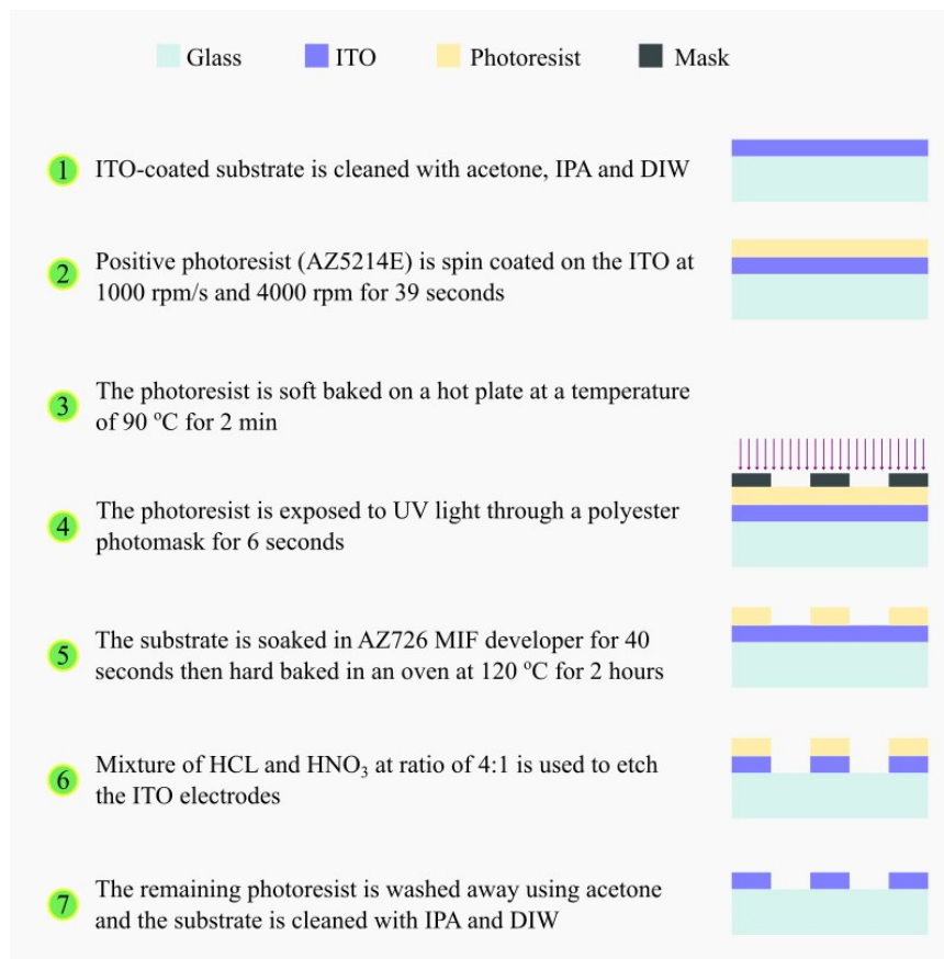
Fig. S1. The steps that are used to fabricate the electrodes of the temperature sensors.
