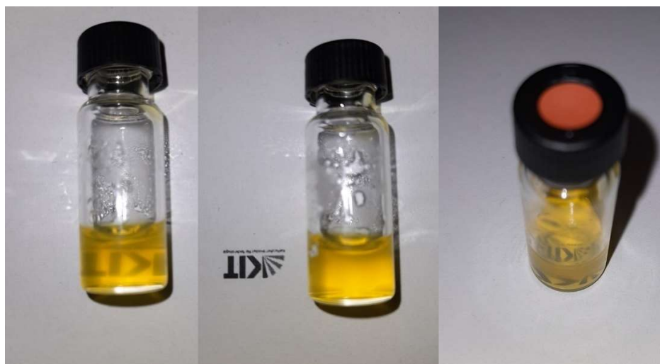
Figure S 6: Pictures of a hydrogel formed by 0.3 wt% gelator 1 and 0.3 wt% alginate (Method B).
