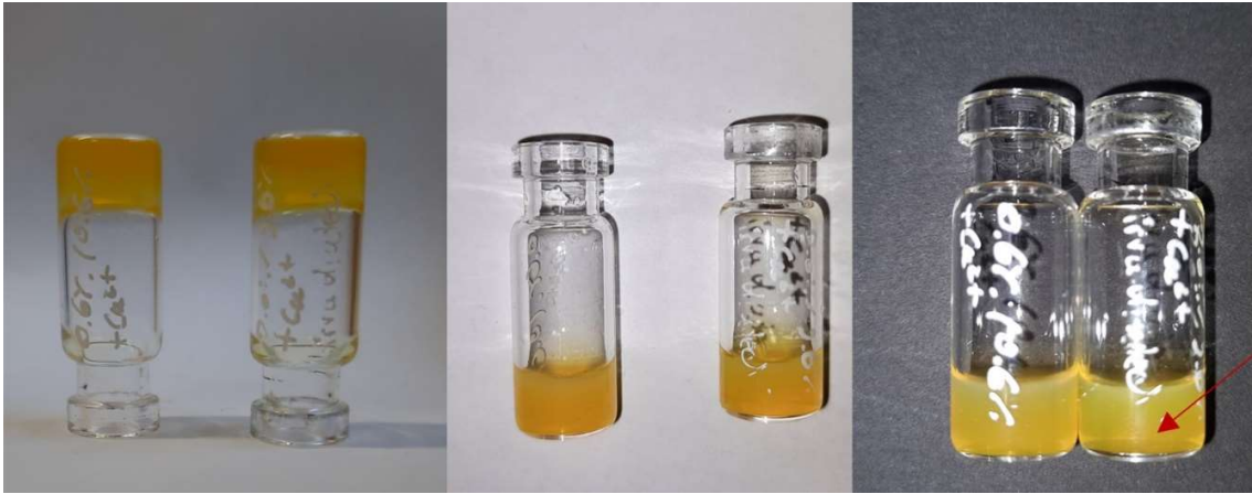
Figure S 13: Remaining gel after the \text{Ca}^{2+} experiment. In each picture the right vial was irradiated. The gel in the irradiated vial is less opaque, the bottom plate of the vial is clearly visible (red arrow).
