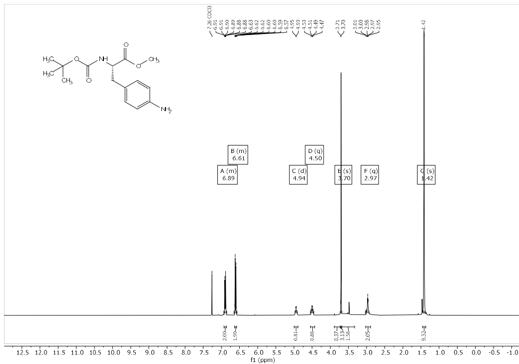
Figure S 27: 1 H-NMR-spectrum (400 MHz, CDCl 3 ) of the compound 5.
