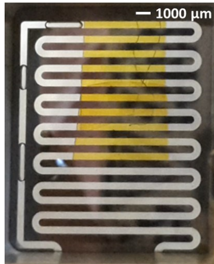
Figure S5. Outgassing occurring at the channel inlet: Large CO 2 bubbles already forming at the inlet of the device (bottom left of the figure).
