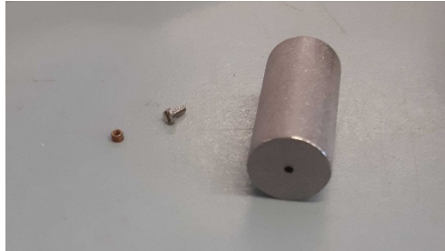
Figure SI 2. Left to right: Image of bushing, screw and filter tip unassembled
