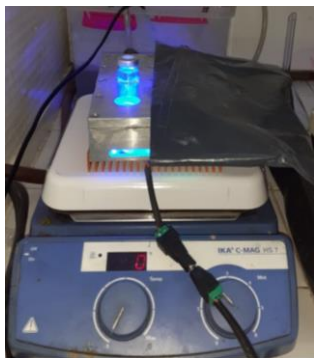
Batch reactor- Blue LED 3 W
