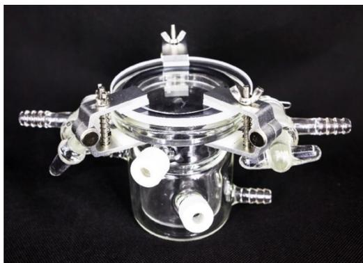
**Fig. S9** Photograph of the photocatalytic  $N_2$  fixation reactor.
