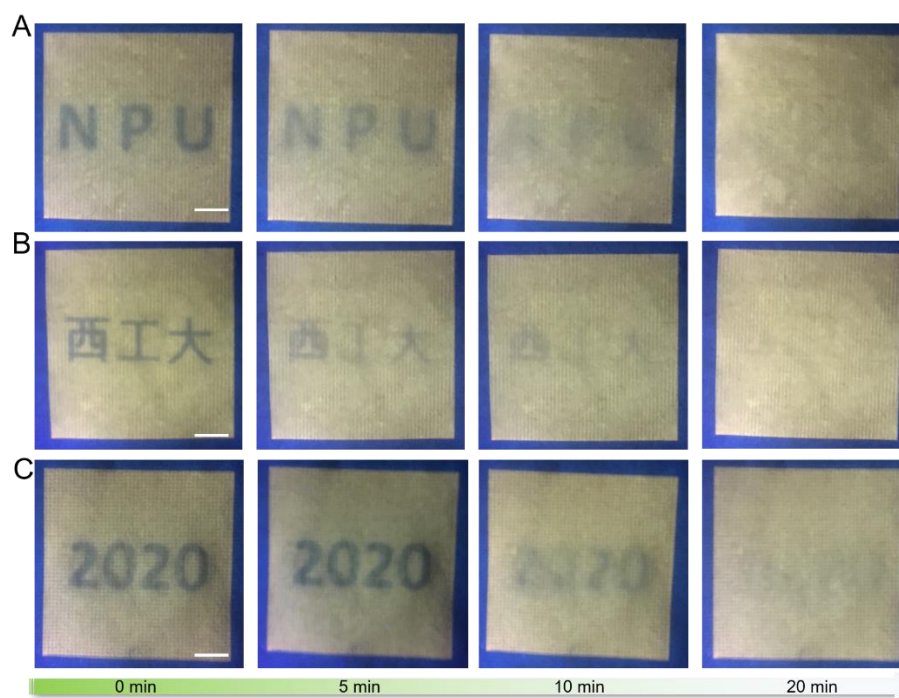
Figure S14. Photographs of the printed patterns derived from 1 , ATP and ALP. The yellow emission background is printed with the aqueous solution of 1 as inks. (A) The “NPU” pattern that printed with the inks of ATP is gradually disappeared after spraying with ALP inks. (B) The reprinted pattern of Chinese characters with ATP inks at the same location of (A), is gradually disappeared after spraying with ALP inks. (C) The reprinted pattern of “2020” with ATP inks at the same location of (B), is gradually disappeared after spraying with ALP inks. [\text{ALP}] = 0.80 \text{ U mL}^{-1} Scale bars: 5 mm.
