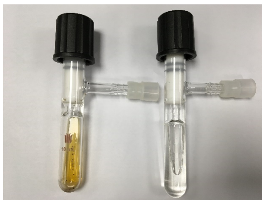
Scheme S1. Bromotrimethylsilane. Freshly distilled one (right); the one after two weeks (left).
