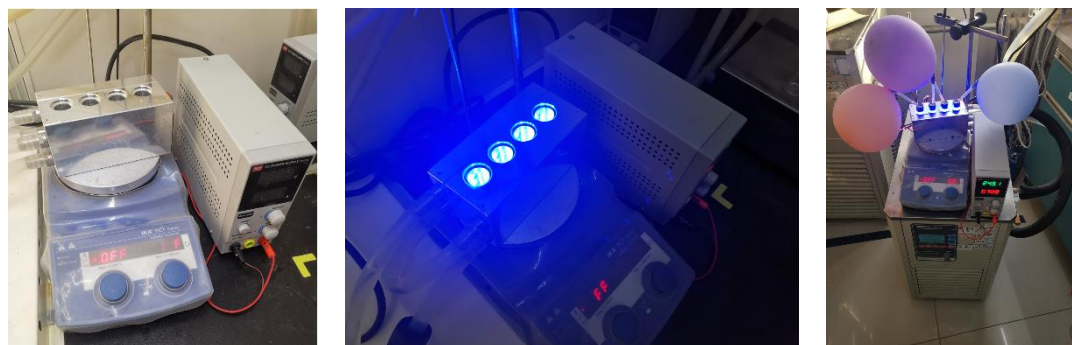
Figure S2: Appearance of Blue LEDs reaction System.
