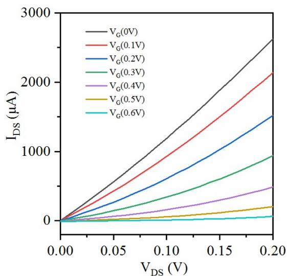
**Figure S2.** Output characteristics of the OEET measured in PBS containing 0.1 M AA after 2000 min.
