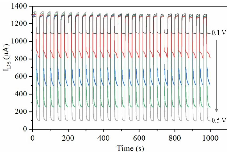
**Figure S3.** The channel current of the OECT measured in PBS containing 0.1 M AA by applying the potential (0.1 V-0.5 V) to Ag/AgCl G-electrode.
