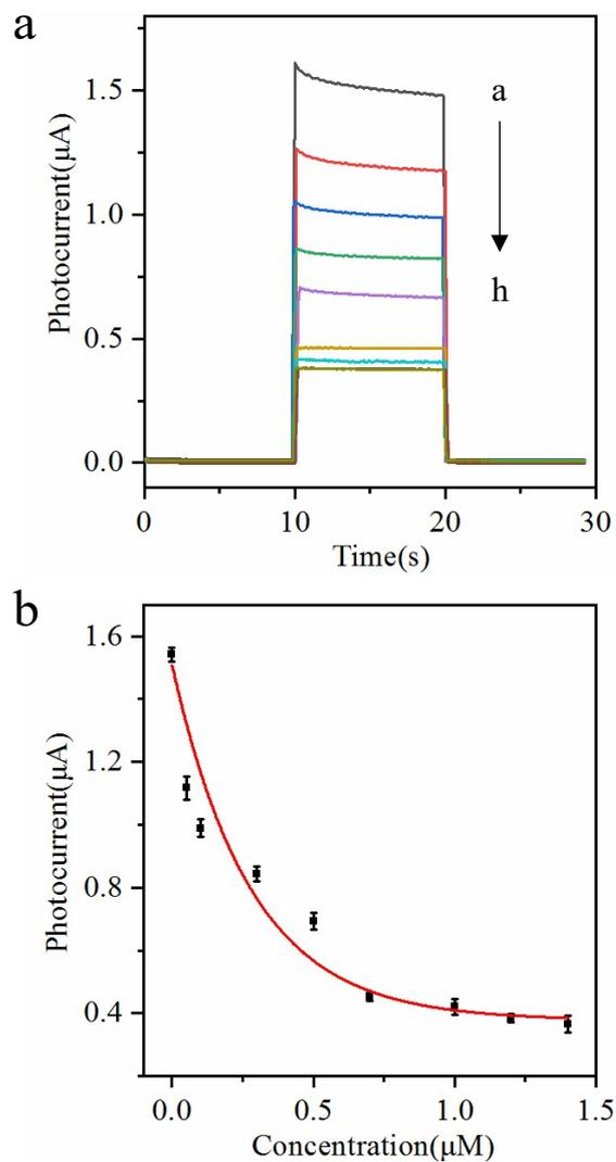
**Figure S6.** (a) Partakers concentrations optimization in traditional PEC bioanalysis and the concentration corresponding to (curves a-h) 0, 0.05, 0.1, 0.3, 0.5, 0.7, 1.0, 1.2, and 1.4  $\mu\text{M}$ , respectively. (b) The corresponding calibration curve.
