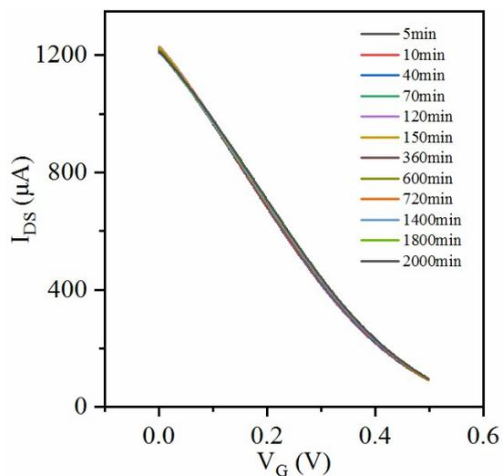
**Figure S1.** Transfer characteristics of an OECT measured in PBS containing 0.1 M AA at different time within 2000 min. G-electrode: Ag/AgCl.  $V_{DS} = 0.1$  V.
