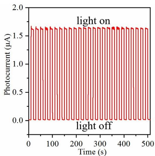
**Figure S4.** Photocurrent stability of CdS QDs/Ti electrode measured in traditional PEC analysis.
