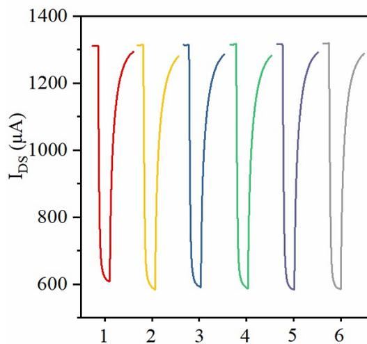
**Figure S8.** The channel current responses of six aptamer/CdS QDs/Ti G-electrodes.
