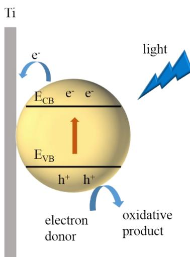
**Figure S7.** Schematic of the charge transfer between CdS QDs and Ti G-electrode.
