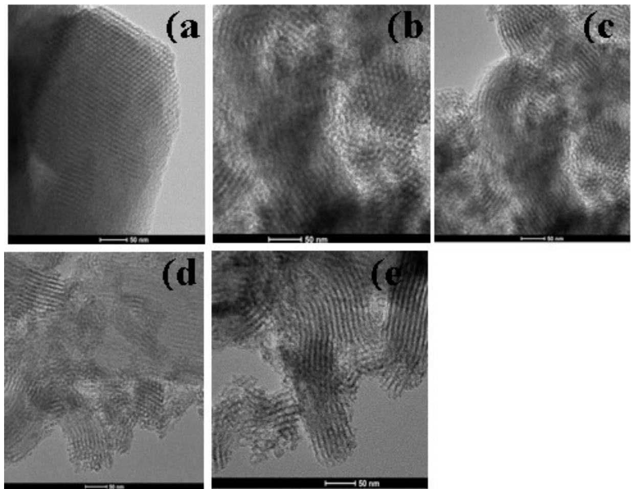
Fig. S1. TEM images of (a) SBA-15, (b) 10%TPA-SBA-15, (c) 20%ZrO<sub>2</sub>/10%TPA-SBA-15, (d) 20%ZrO<sub>2</sub>-SBA-15 (e) 10%TPA/20%ZrO<sub>2</sub>-SBA-15.
