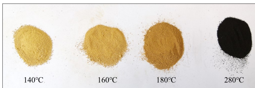
Figure S2. Solids after HTL in different temperatures (10/100 g/mL, 60min, ethanol)
