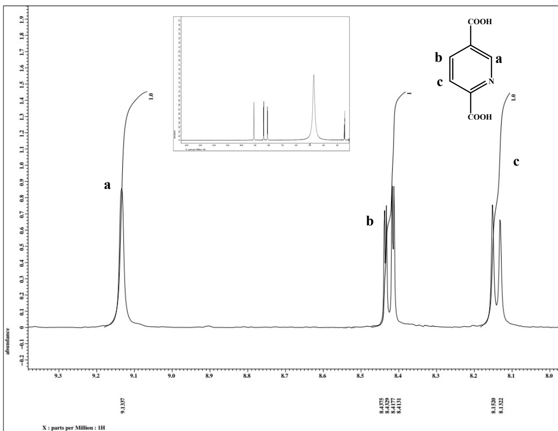
Fig S21. ^1\text{H} NMR spectrum of 2,5-PDCA recovered digesting Al-PDC in conc. HCl. Full spectrum is inset
