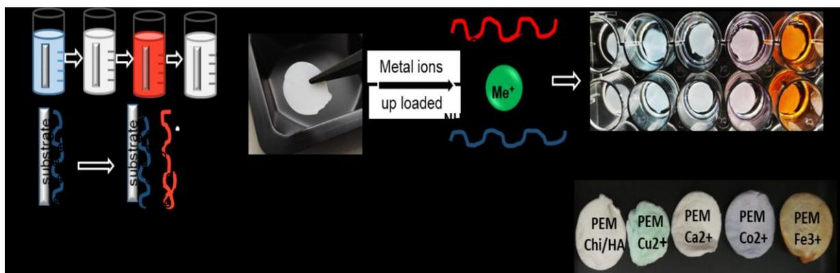
**Figure S2:** Scheme of freestanding multilayer film preparation with subsequent crosslinking with high concentrations of metal ions and photographs of the resulting films with obvious staining by the metal ions.
