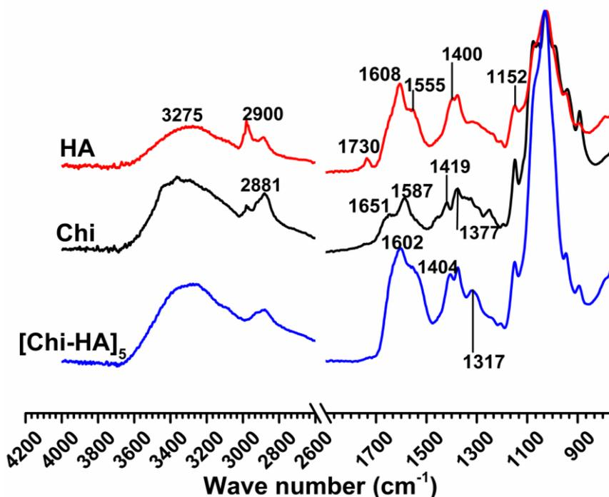
**Figure S3:** FTIR spectra of pure chitosan (Chi), hyaluronic acid (HA) and dry [Chi/HA]<sub>100</sub> multilayer films
