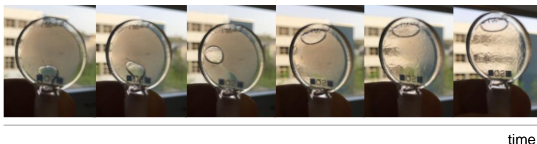
Figure S4. Pictures of CPEG 6k / ethanol (2 wt%) cooled at -60\text{ }^{\circ}\text{C} and then exposed to air to see how the solid-like paste evolve in about 1 min. First, the liquid starts to move (the bubble moves up) and then, the turbidity disappears. Droplets in the cuvette glass are due to water condensation.
