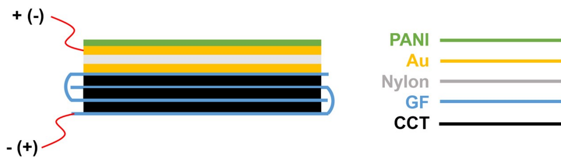
Fig. S8 Cross-section schematic of the layered structure of PCECD.
