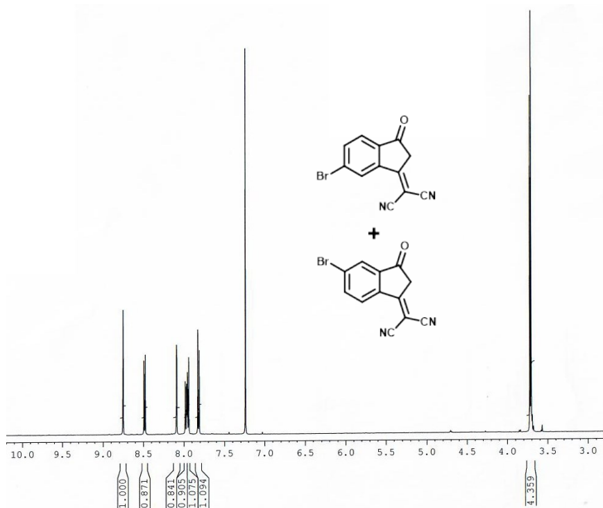
Figure S2. ^1\text{H} NMR spectrum of 2-(5(6)-bromo-3-oxo-2,3-dihydro-1 H -inden-1-ylidene) malononitrile in \text{CDCl}_3 .
