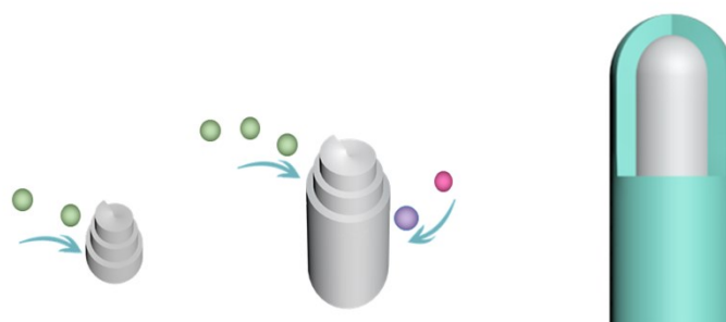
Figure S1. Schematic illustration of the axial screw dislocation-driven growth mechanism of Zn@Ni-P NWs.
