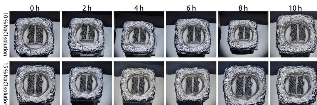
**Figure S19.** Optical images of salt precipitation on the surface of CCMF-4 in 10% and 15% NaCl solution.
