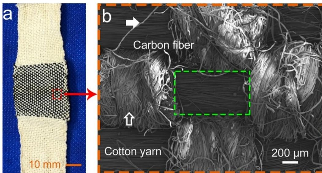
**Figure S7.** (a) Optical images of CCMF-1. (b) The SEM image of the obtained CCMF-1. The solid arrows and hollow arrows indicate carbon fiber bundle and cotton yarn, respectively.
