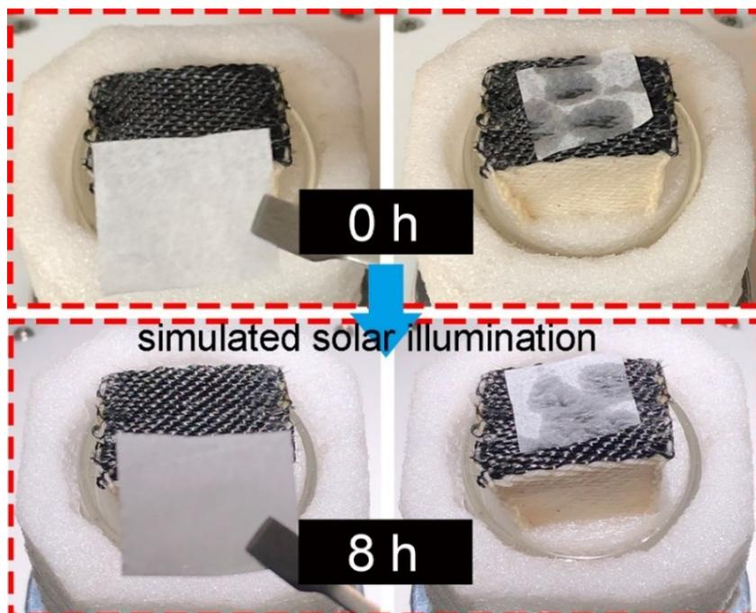
**Figure S12.** The tissue paper placed on the top of CCMF-4 can be wetted before and after 8 h illumination under 1 sun.
