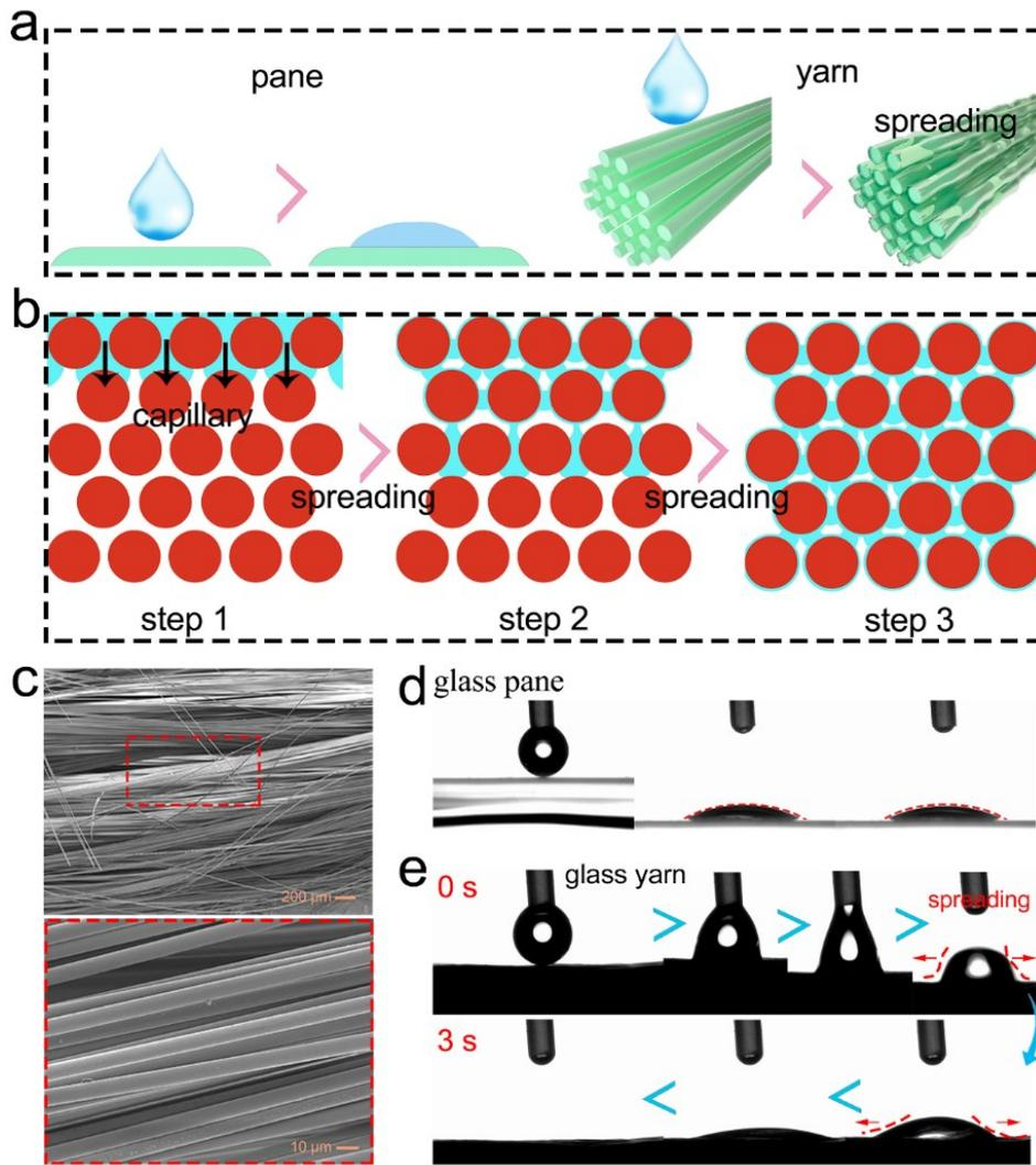
**Figure S4.** (a) Schematics showing that the water spreading on the pane and yarn when water drop contacts the corresponding surfaces. (b) A series of cross-sectional views showing the dynamic formation of the water wetting process on yarn. (c) SEM images of glass fiber yarn. The water contact angle of glass pane (d) and glass yarn (e).
