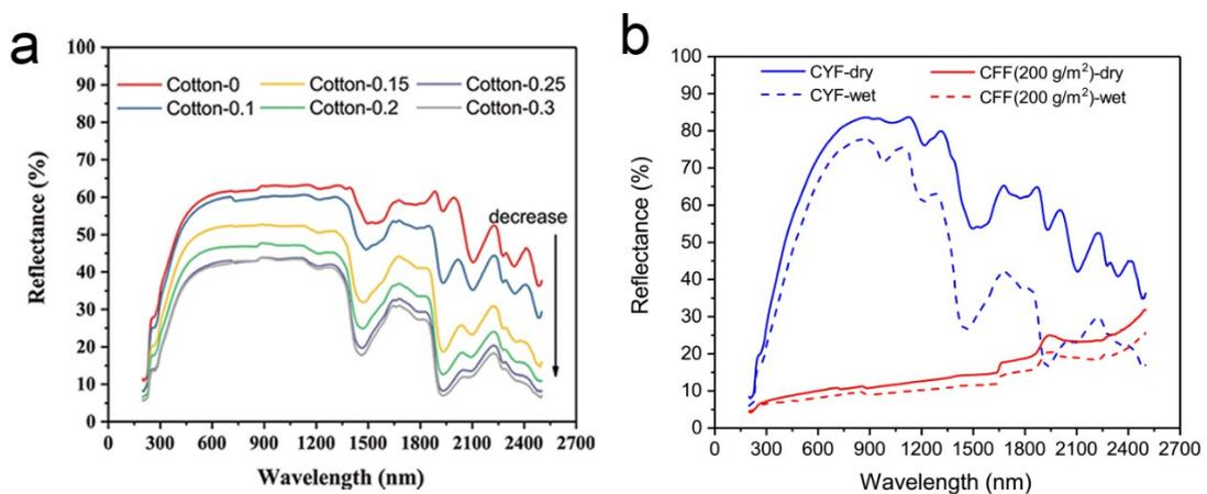
**Figure S5.** (a) Reflectance spectra of the wet cotton fabric in the wavelength range of 250~2500 nm (cotton-X is regarded as cotton fabric with different water weight (X) in volume (ml)). (b) Reflectance spectra of the wet and dry CYF and CFFs in the wavelength range of 250~2500 nm.
