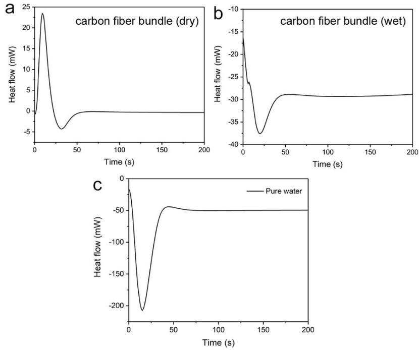
**Figure S6.** DSC spectra of carbon fiber at (a) dry and (b) wet state in the temperature range from 25 to 40 °C. (c) DSC spectra of pure water in the temperature range from 25 to 40 °C.
