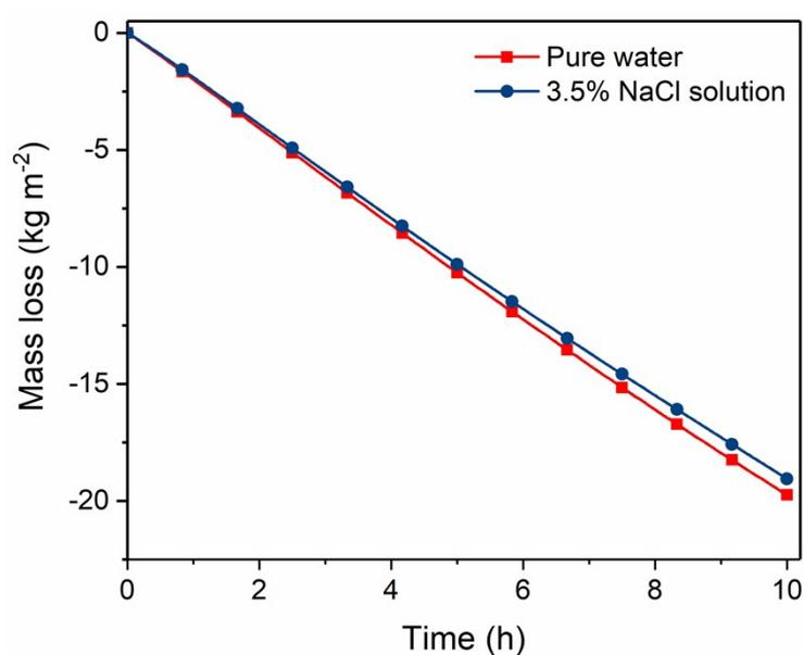
**Figure S18.** Mass loss of pure water and 3.5% NaCl solution through CCMF-4 under 1 sun illumination as a function of time (10 h).
