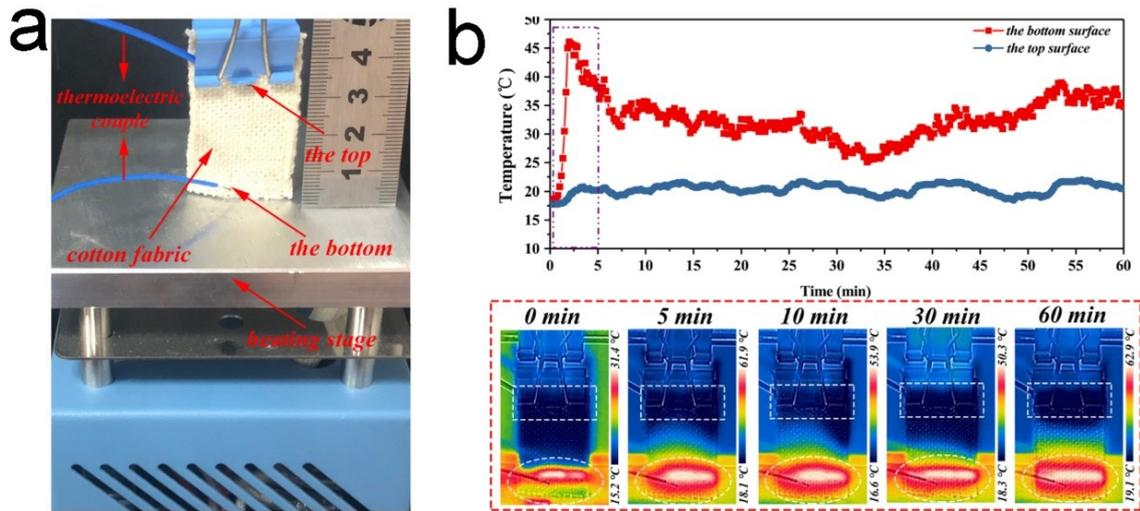
**Figure S9.** (a) The optical image of a device for the property of thermal conductivity of cotton yarn fabric. (b) The real-time temperature of the top and bottom of cotton yarn fabric in the warp direction. (c) The corresponding infrared images.
