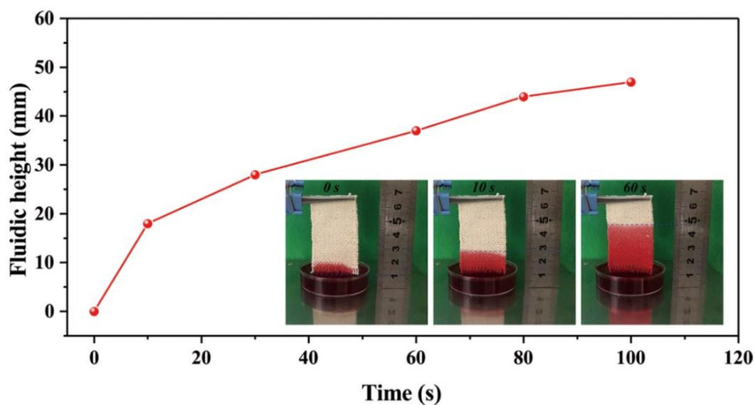
**Figure S8.** The rate of fluidic transport of cotton yarn fabric in the warp direction.
