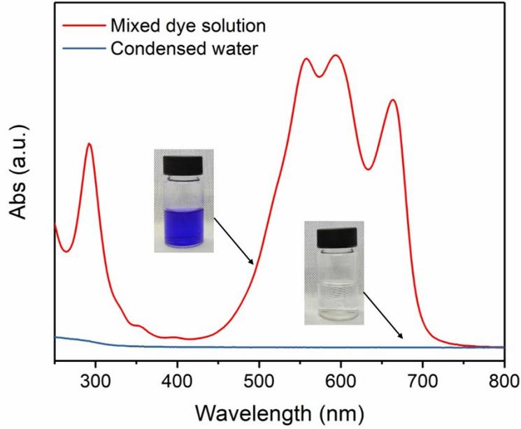
**Figure S20.** UV–vis absorption spectra of mixed dye solution and the condensed water through steam. The insets show the corresponding optical photos.
