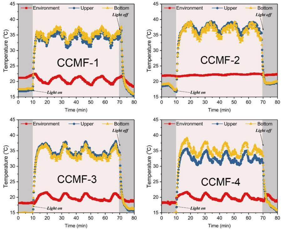
**Figure S15.** Temperature changes of CCMFs resulting from switching 1 sun illumination on and off.
