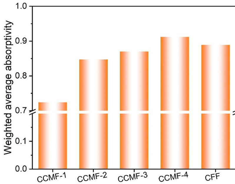
**Figure S10.** The weighted average absorptivity of various samples in solar spectrum region (280-2500 nm).
