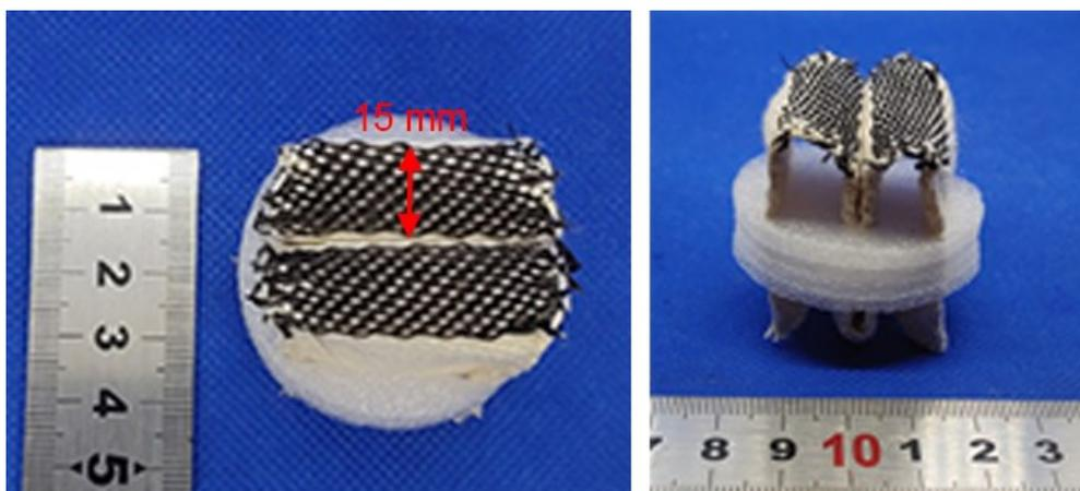
**Figure S17.** Optical image of CCMF-4 based solar generation device with salt resistance.
