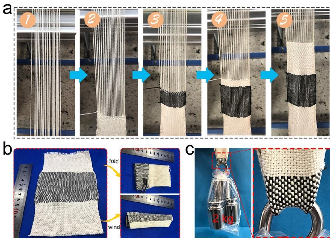
**Figure S1.** (a) Optical images of the fabrication process of CCMF-1. The flexibility (b) and mechanical property (c) of CCMF-1.
