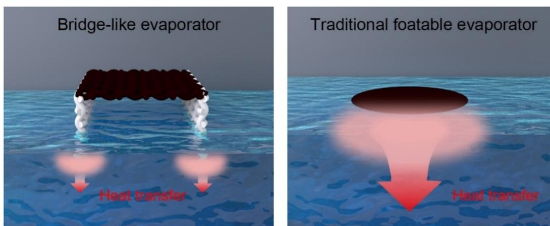
**Figure S13.** Schematic illustration of heat loss of bridge-like evaporator and traditional evaporator. Heat loss can be controlled by minimizing the contact area with the bulk water in a bridge-like evaporator.
