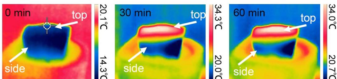
**Figure S14.** Side and top view of Infrared images of the CCMF-4 based evaporator under 1 sun.
