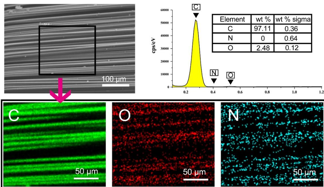
**Figure S2.** Elemental composition (C, O, and N) and (c) maps of carbon fiber bundle.
