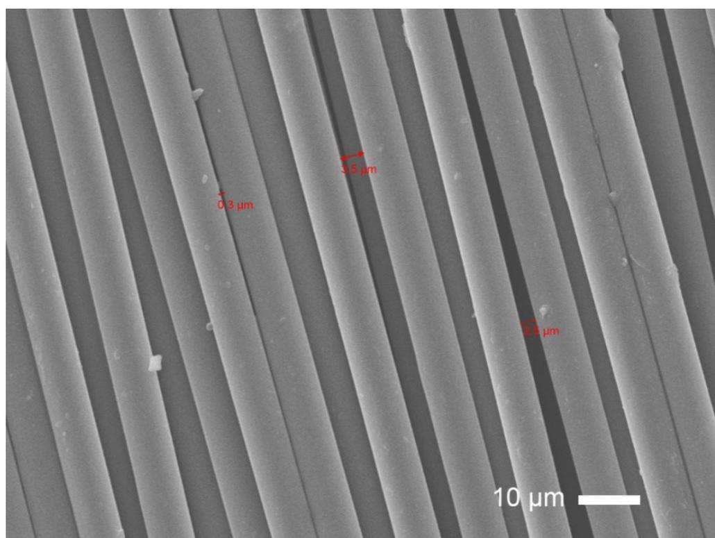
**Figure S3.** The size of the gap between the adjacent carbon in carbon fiber bundle.
