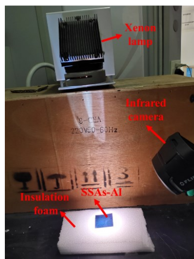
Fig. S11. The device diagram of photothermal experiment for ANEAC SSAs under standard solar radiation.
