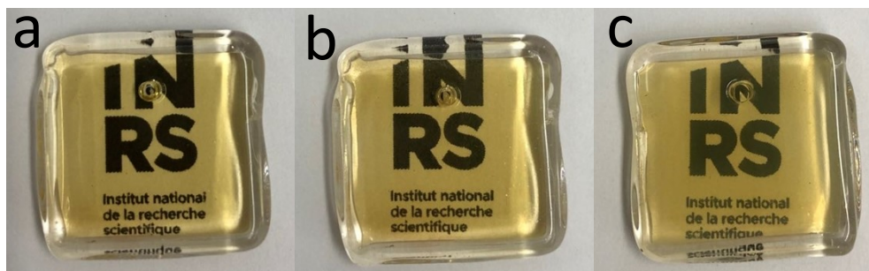
Fig S7. Liquid LSC fabricated with quartz cells: (a) Bare Cdots, (b) Cdots + Ag40@SiO 2 , (c) Cdots + SiO 2
