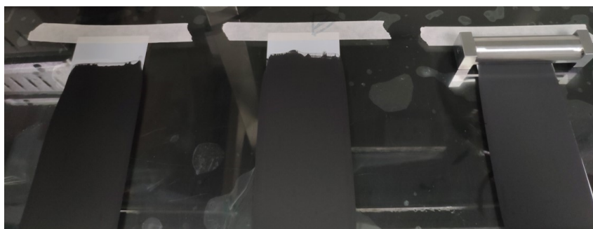
Figure S6. Photograph of the typical coating process for preparing CNMCO/PP separator.
