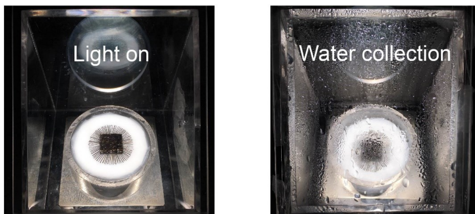
Fig. S26 Optical images of the solar desalination prototype and water collection situation treating the artificial seawater with 3.5% salinity.
