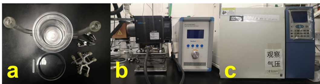
361 Figure S19. Digital photographs of (a) glass reactor, (b) 300 W xenon lamp with the 362 model of PLS-SXE300C and (c) gas chromatography for H 2 evolution system.
