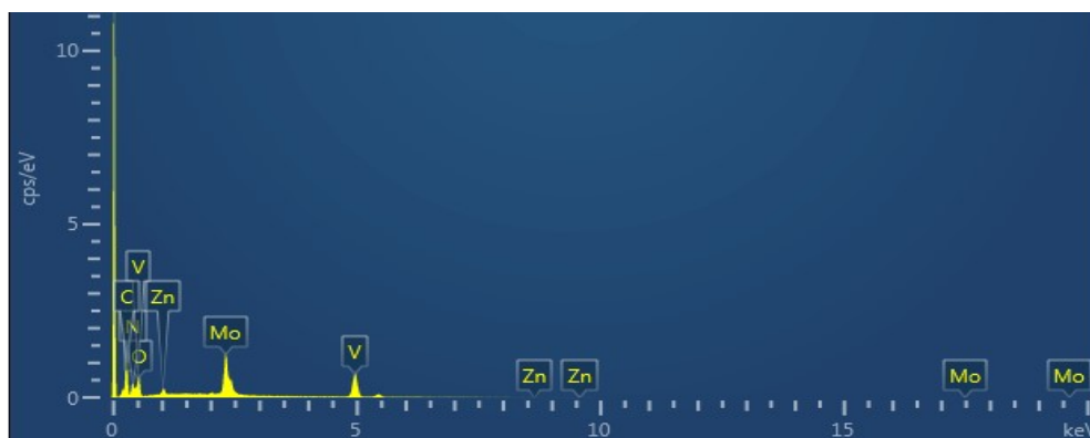
Figure S21. EDX spectrum of the CC@a-MVO/MVN cathode at full charge.
