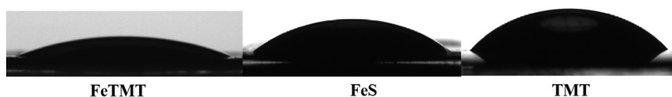
Fig. S14. Real wastewater contact angle of the FeTMT ( 26.2^\circ ), FeS ( 36.0^\circ ), TMT ( 42.6^\circ ).
