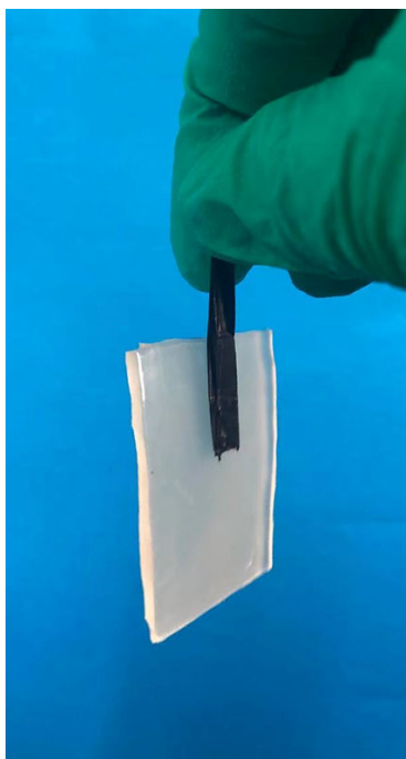
Fig. S13 Good adhesion between CNTs film current collector and hydrogel electrolyte due to hydrophilic interaction and hydrogen bonding.
