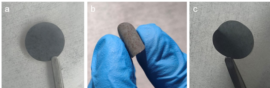
Figure S9. Photographs of a BIG electrode containing Cu substrate (a), the BIG electrode under bending (b) and after bending (c).
