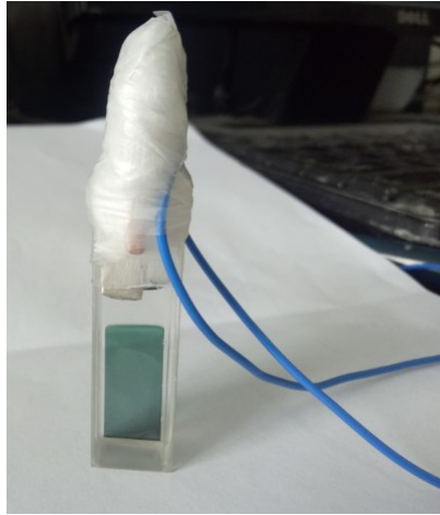
Figure S3. The schematic diagram of microelectrochemical cell open lithium battery test
