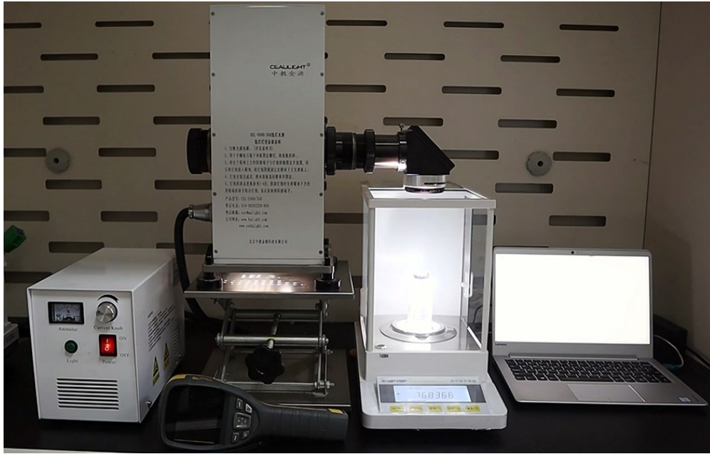
Figure S8. The optical image for solar-driven evaporation measurement platform.
