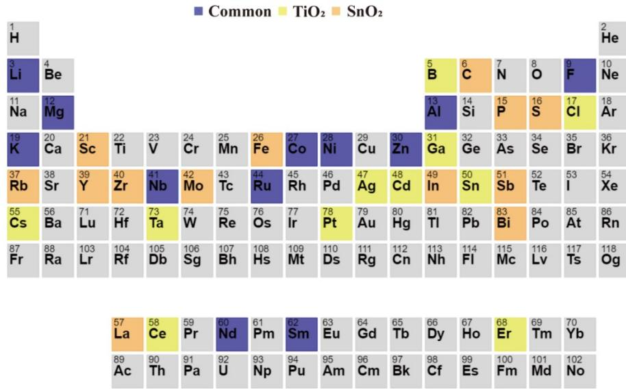
**Figure S1.** Doping elements used for the  $\text{TiO}_2$  and  $\text{SnO}_2$  ETLs. Some elements are doped only in  $\text{SnO}_2$  or  $\text{TiO}_2$ , while some other elements are doped in both.
