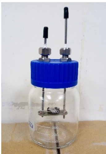
Fig. S11 Specially designed bottle for electrochemical tests of Li–gas batteries.
