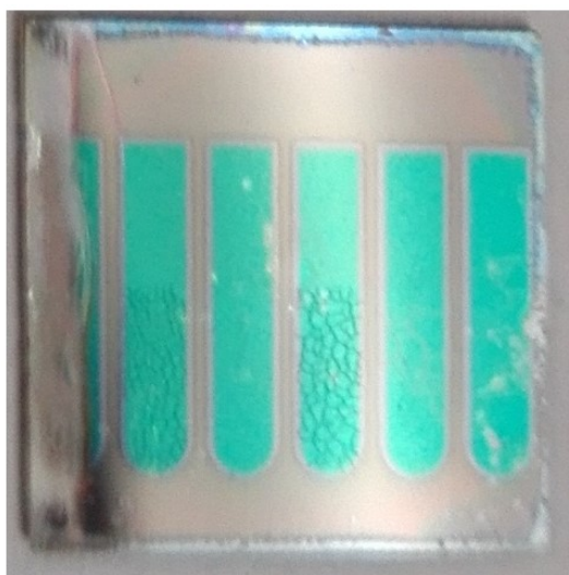
Fig. S3 Photograph of perovskite solar cells with \text{SnO}_2 buffer layer and IZO electrodes deposited at a target-substrate distance of 10 cm after cooling to -5^\circ\text{C} .
