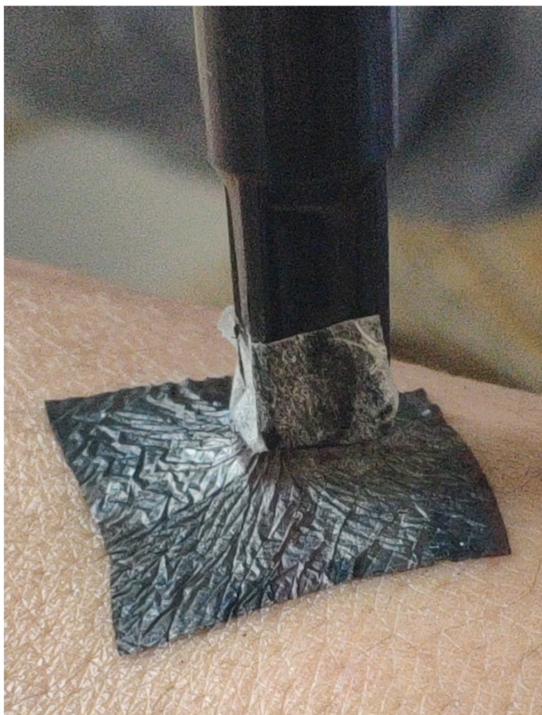
Figure S6. The nanomesh-reinforced graphene pulled by the force of 0.2 N with the stress area of 0.28 cm 2 .
